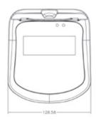
5VDC at 150mA 120V AC adapter or USB host terminal port RS-232, Baud rate from 1200 to 115200 USB CDC, 2.0 Full Speed
